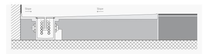
The highly efficient Joulia-Twinline DWHR is not only available as a stainless steel channel drains, but can also be combined with shower surfaces made of solid surface material.
